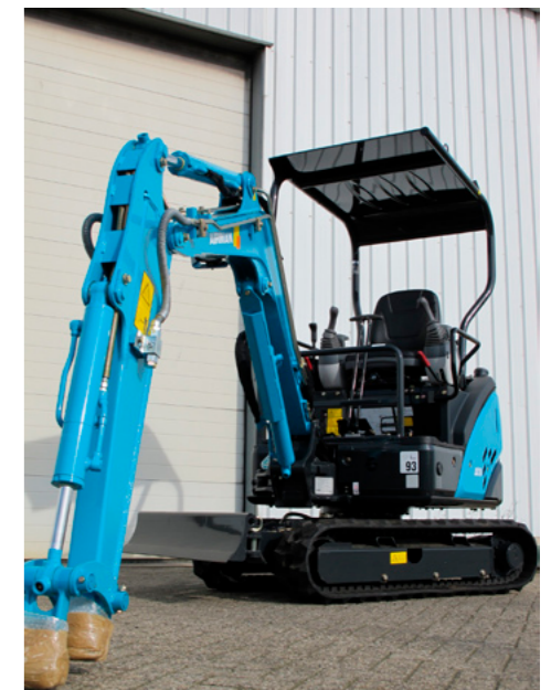
AX18-4 equipped with a 3 pole canopy which can easily be removed by only taking out 7 bolts.
