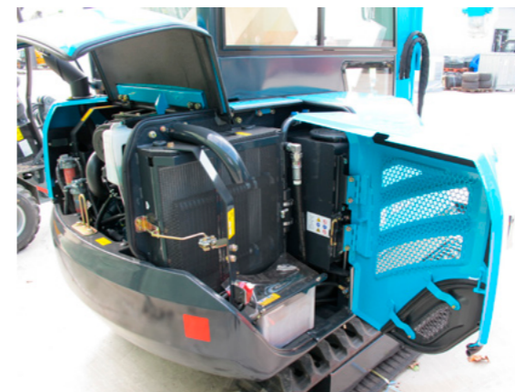
Wide to be opened covers for quick maintenance (AX27-3 pictured)
